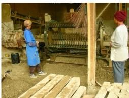
On emerging form the brick-cutting process, the 'green bricks' are removed from the conveyor and stacked to dry.
